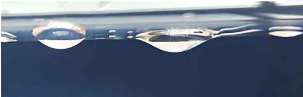
Quartz glass sleeve without T-Tauri coating
